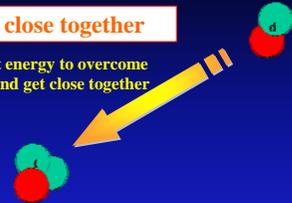
Heat the plasma to a very high temperature, so that the kinetic energy of the nuclei is high.
