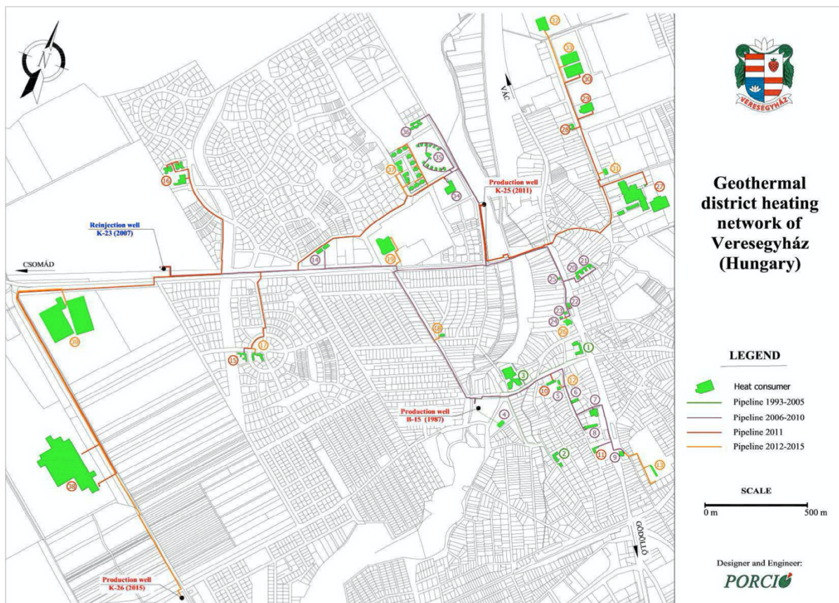
Figure 15. Geothermal wells, pipelines and heat consumers in Veresegyház in late 2016. Refer to numbers in Table 3 for identification of heat consumers. Source: Szita (2016) 47
