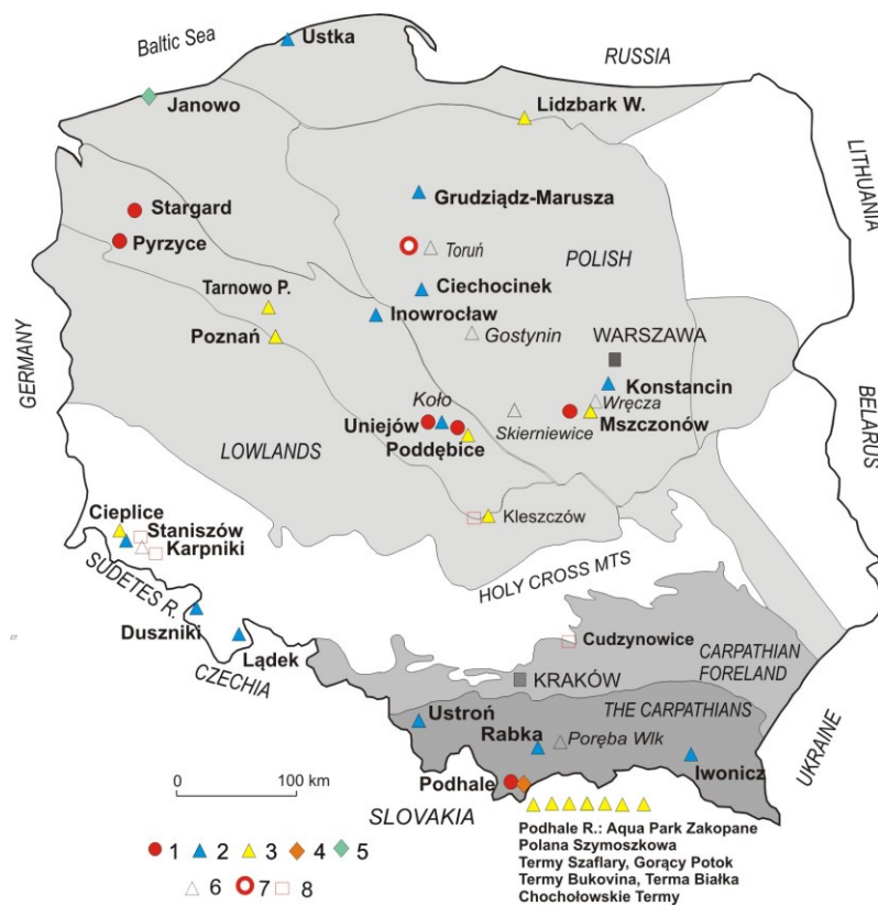
Figure 29. Geothermal energy projects in the Poland Lowlands (light grey area) and the rest of Poland in late 2018: 1. district heating plants, 2. health resorts, 3. recreation centres, 4. wood drying, 5. fish farming, 6. recreation centres in development, 7. district heating systems in development, 8. individual heating systems. After Kępińska (2020) 86
