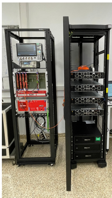
Figure 22. SABRE DAQ electronics (left) and server units (right).
