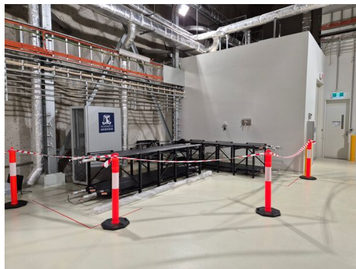
Figure 17. Muon detectors in SUPL, assembled in ‘telescope’ mode, which is the configuration required to measure the muon flux and angular spectrum (from two directions). Reproduced with permission from [68].
