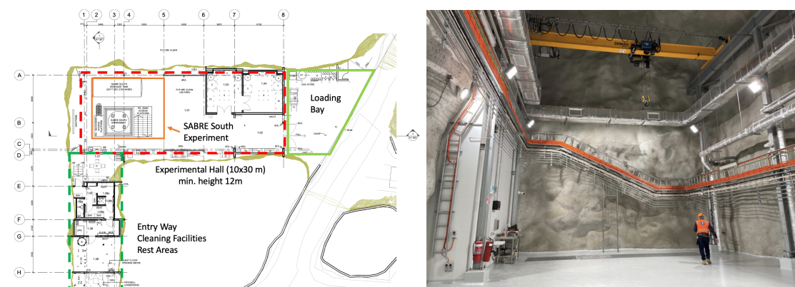
Figure 3. Left: schematic of SUPL including the main experimental hall (top left), low background counting (HPGe) facilities (top middle), loading bay (top right), and the entry way with cleaning facilities (bottom left). Right: photograph of SUPL. SABRE South will be located near the centre of the image. The door on the left leads to the rest areas and entry way.
